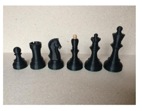
An important factor in getting a smooth finish on your pieces is to randomise the start points for each layer. In Simplify 3D this setting is in the FFF settings, layer tab. Random start points ensures that oscillations caused by your printer do not repeat vertically along the model. This slightly increases the print time but results in much smoother vertical surfaces.
